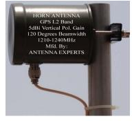
polarization diversity (Optional). The HR-1227-5 Horn Antenna is light weight, broadband and rugged horn antenna, ready mobility, easily mounts, supplied with fiberglass radome to protect the antenna from environment. N-Female output termination of horn antenna is fixed directly at the wall of horn antenna. All the screws, nuts and bolts of horn antenna are made of marine grade stainless steel.
