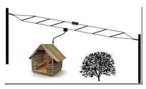
configuration (Horizontal Polarized) using two masts. The HF Broad Band Dipole Antenna provides optimum performance over complete HF band, eliminating the requirement of multiple antennas or an Antenna Tuning Unit.
