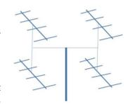
as matching device to keep the VSWR low resulting in increased efficiency of the dual yagi antenna. The antenna can be mounted to obtain any horizontal or vertical polarization. Similarly the antenna can be stacked either horizontally, vertically or in a square configuration to control the beam-width in desired plane.
