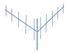
CONSTRUCTIONS: Radiating elements and supporting booms of dual yagi antenna have been constructed in high quality 6063T6 ultra corrosion resistant architectural aluminum alloys to prevent
