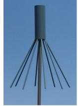
and all fasteners are made of stainless steel. Large diameter vertical radiating element ensures the constant vertical beam-width of 76 degrees and 2dBi gain over the entire band. Antenna termination and feed cable lie enclosed inside the mounting pipe for complete weather protection.
